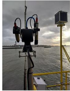
Hyperspectral autonomous radiometer system (PANTHYR) on RT1 platform
