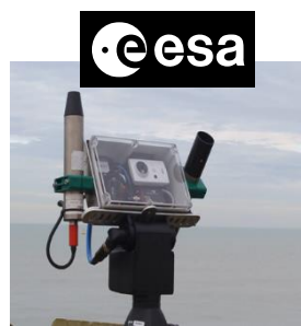
PANTHYR system [Vansteenkoven et al, 2019] 400-900nm, 10nm FWHM
