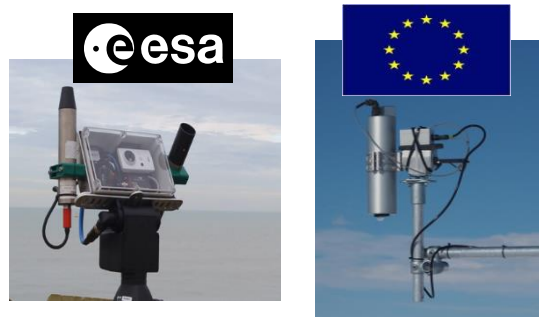
PANTHYR system [Vansteenkoven et al, 2019] 400-900nm, 10nm FWHM
